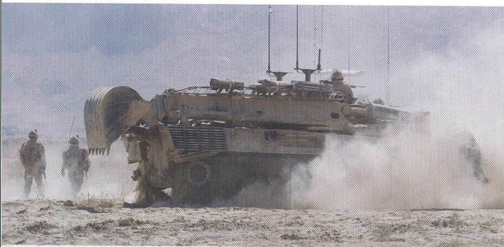
The Badger armoured engineer vehicle, based on the Leopard 1 chassis, will be replaced by up to 18 AEV derivatives of the Leopard 2 under the Force Mobility Enhancement project. (Photo: DND)
