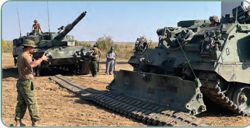
MCpl Lapid guides Cpl Aberle in the ARV to flip track during Ex Steele Sabre 23
