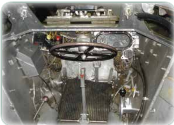
Driver compartment of a Ferret armoured car.
