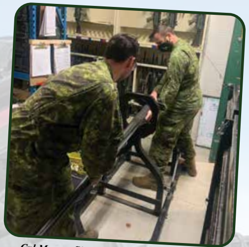
Cpl Marcus Skafar and Cpl Connor Cantwell run a gauging device to determine serviceability of a 25mm Bushmaster.
