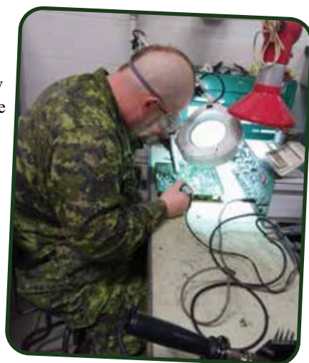
Cpl Wesley Smith performs soldering repairs on a printed circuit board.
