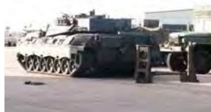
A Leopard C2 after the turret was replaced.
